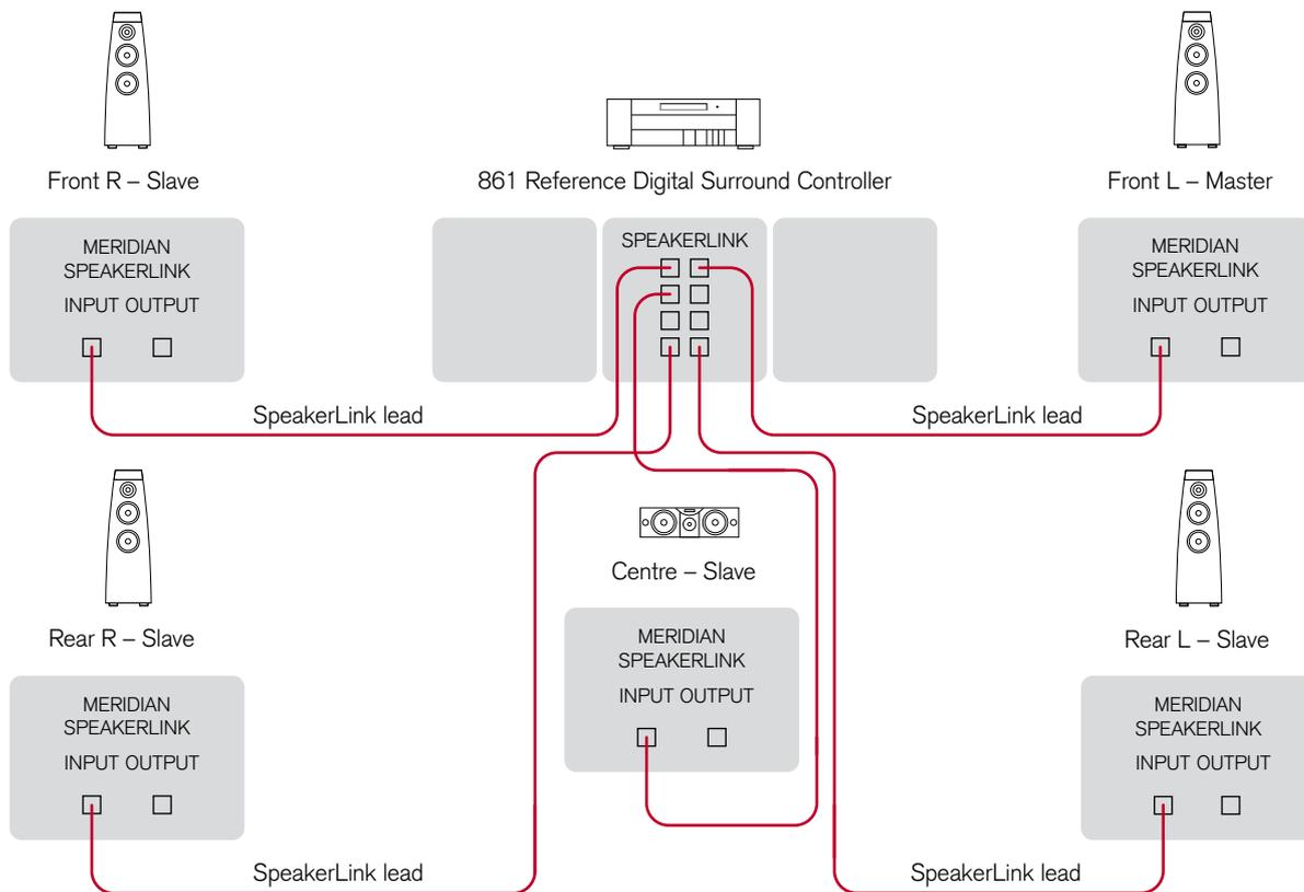
This is an alternative to the “daisy chain” wiring configuration shown opposite.
