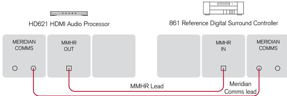
The 861 provides an MMHR multichannel input which can be used with the HD621 HDMI Audio Processor.
