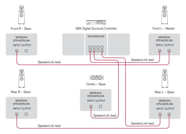
This is an alternative to the "home run" wiring configuration shown in the next section.
