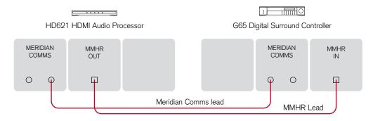
The G65 provides an MMHR multichannel input which can be used with the HD621 HDMI Audio Processor.
