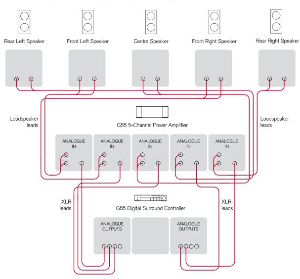
The G65 provides eight balanced analogue outputs to allow you to connect to active loudspeakers, or power amplifiers and passive loudspeakers. An ideal choice is the Meridian G55 5-Channel Power Amplifier.
