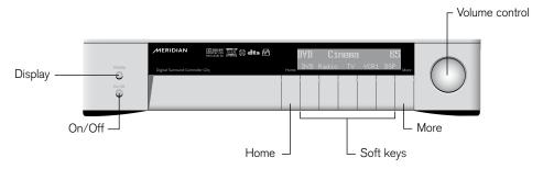
The five soft keys under the display make the G Series products particularly easy to use. They change to reflect what the product is doing. For example, if you are customizing the DSP settings they provide controls to label and store the preset. The current function of each key is shown above the key on the bottom line of the display.
