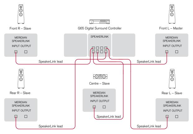
This is an alternative to the "daisy chain" wiring configuration shown in the previous section.
