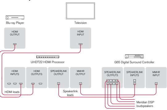
This is an audio-visual system with a Blu-ray player, and a surround system based on five Meridian DSP loudspeakers controlled by a Meridian G65 Digital Surround Controller. If the television supports CEC the G65 can receive the television sound via the HDMI connection using ARC.
