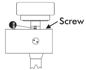
Slacken off the screw just enough to be able to revolve the arm tube without applying force. Note! Do not remove the screw completely!
