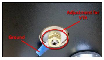
Loosen the nut under the tone arm-base, remove the ground wire, then you may adjust the height by turning the brass nut.
